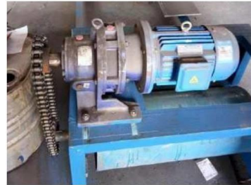
电机、减速机、链条链轮 Motor, reducer, chain sprocket
