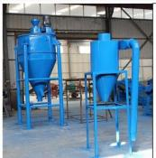
Function: used to separate the fiber impurities, nylon from both nylon waste tire and steel wire tires
