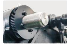
High-precision gear-based mold adjustment mechanism ensures stability and part quality
