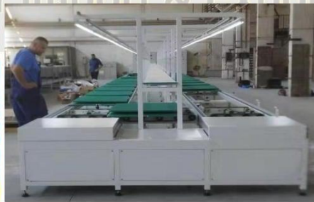
Annular Pallets Assembly Line
